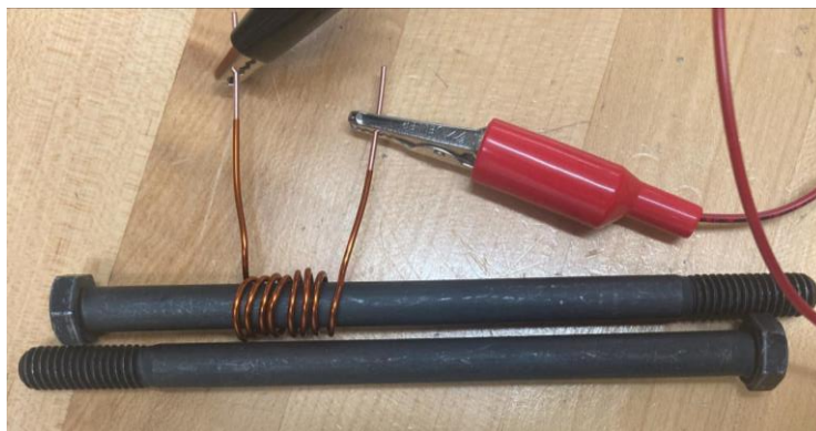
Figure 9: Placement of the coil next to the second bolt as instructed in step 4 of this procedure.
