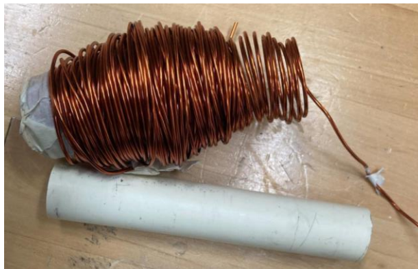
Figure 26: The coil is removed from the PVC pipe and the paper is extracted using the instructions from step 1 of this procedure.
