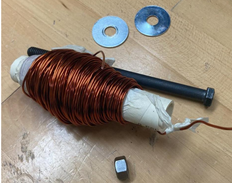
Figure 25: After completing step 5 of this procedure, the PVC pipe, bolt, washers, and nut should all be disassembled and separate.
