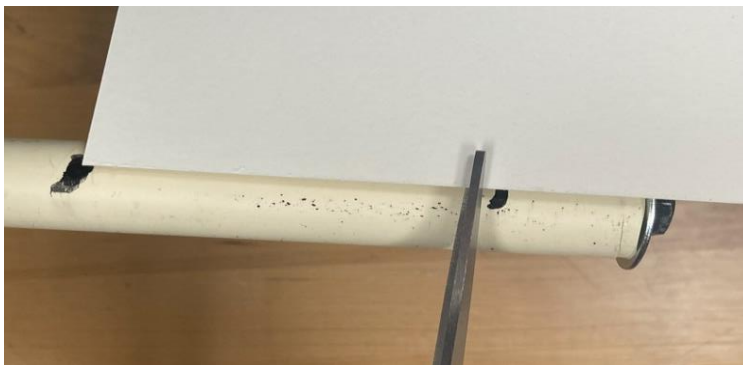
Figure 19: As explained in step 3 of this procedure, use a pair of scissors to cut the provided paper into a strip that fits between the two marks on the PVC pipe.
