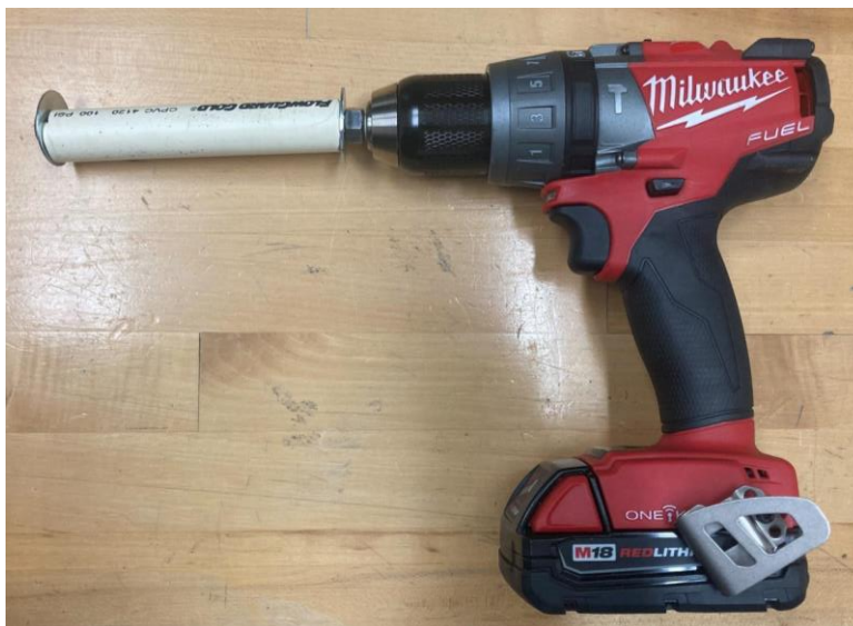
Figure 23: The bolt setup from step 1 of this procedure is inserted into the drill using the instructions from step 2 of this procedure.
