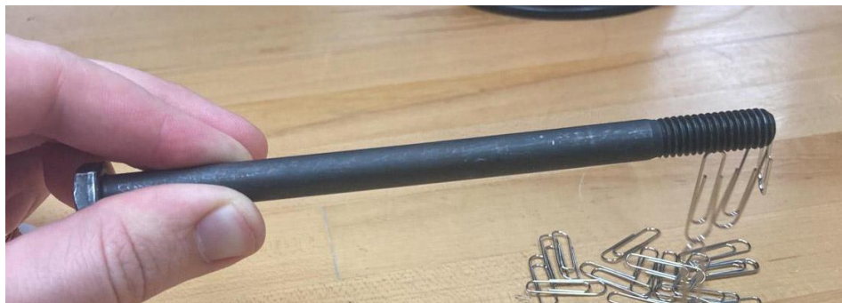
Figure 14: A magnetized bolt picking up several paper clips, the result of step 12 of this procedure.
