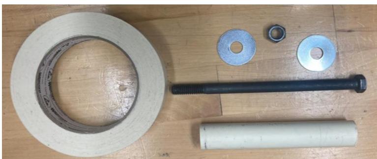
Figure 21: The materials necessary for option two include masking tape, a bolt, a PVC pipe, two washers, and a nut.
