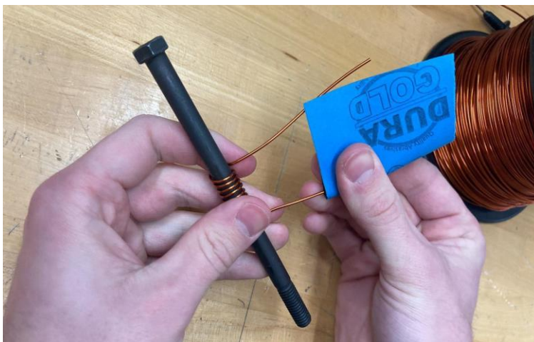
Figure 5: The sandpaper is used to rub off the insulating layer of the wire described in step 2 of this procedure.
