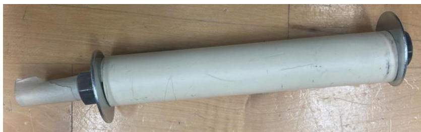
Figure 22: The result of step 1 of this procedure is a bolt with a PVC pipe sandwiched between two washers and secured using a nut.
